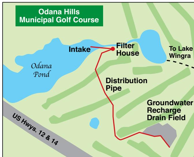
The amount of water withdrawn is about one third of what typically flows through the pond from the upstream watershed. The outfall level of the pond has been raised by six inches, holding back water to be used for infiltration. The median pond level and the shoreline are expected to be the same as before the project. The pond should have more stormwater retention capacity during rainfalls.
