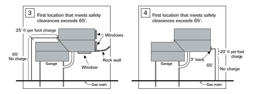
Measurement is to the riser, not the outlet of the meter bracket.
