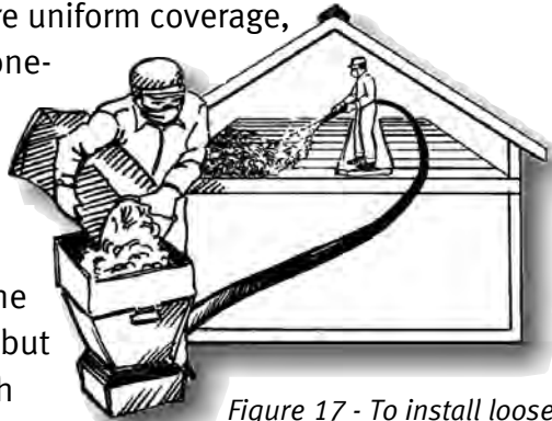
Figure 17 - To install loose-fill insulation, one person fills the blowing machine while the other directs the insulation into the attic.
